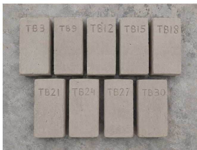
Figure 1. General appearance of bentonite-based brick specimens dried under natural conditions
