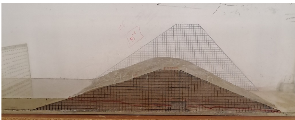
Figure 3. Wetting zone and phreatic surface observed in the laboratory earth dam model
