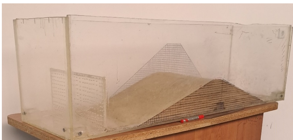
Figure 1. General view of the transparent hydraulic flume and the earth dam model
