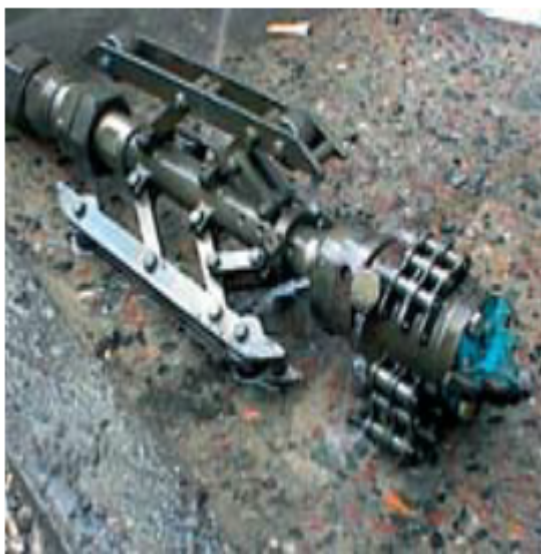
Figure 1.2. Pipeline cleaning equipment with brush or chain drives
