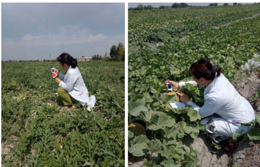
Figure 1. On-site nitrate screening of melon and watermelon samples using a Greentest Eco 3F portable nitrate analyzer
