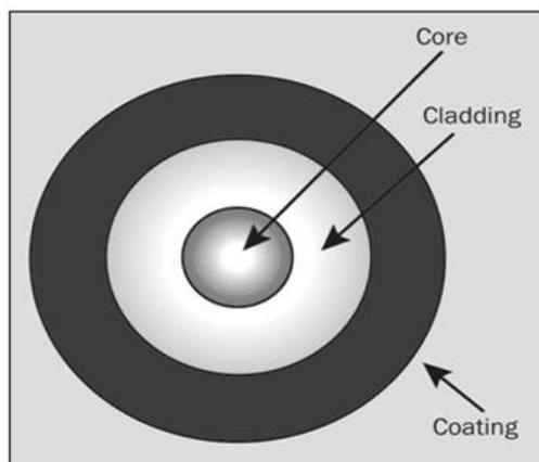
*Figure 1. An optical fiber consists of a core, cladding, and coating*
