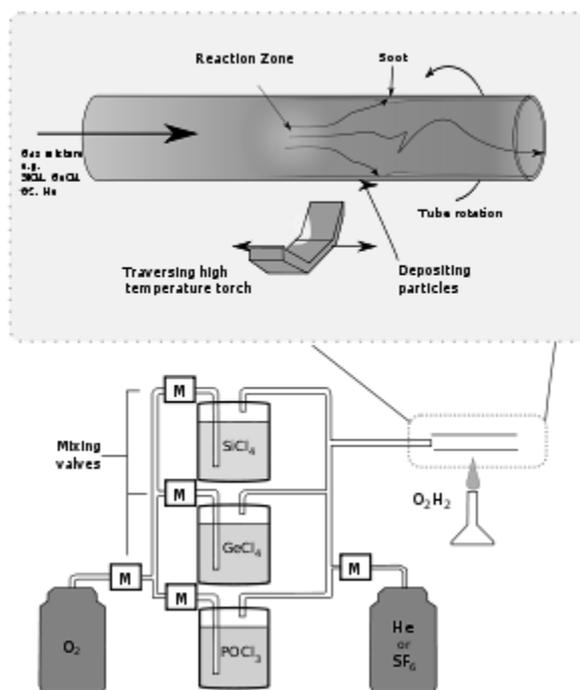
Figure 2. Illustration of the modified chemical vapor deposition (inside) process
