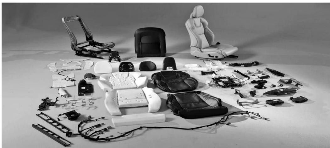
*Picture 1. The Volvo XC90 seats show how something perceived as a solid object turns out to be a complex construction with many parts to make [2]*
